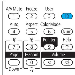
2. While holding the ID button, press the numbered button on the remote control (1 through 9) that corresponds to the ID of the projector(s) you want to operate. Selecting zero lets you control all projectors.
