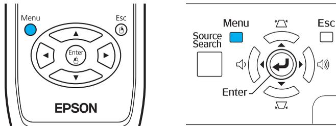
From the Setting menu, select **Keystone** and press **Enter**. Use the
