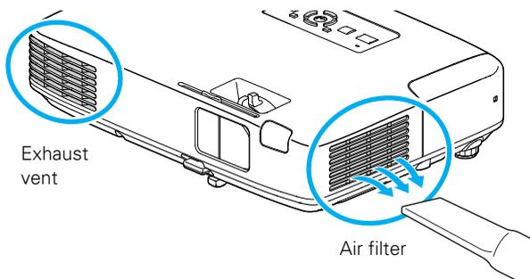
3. If the dirt is difficult to remove or the filter is broken, replace the filter as described on page 72. Contact your dealer or call Epson at 800-GO-EPSON (800-463-7766) to obtain a new filter.
