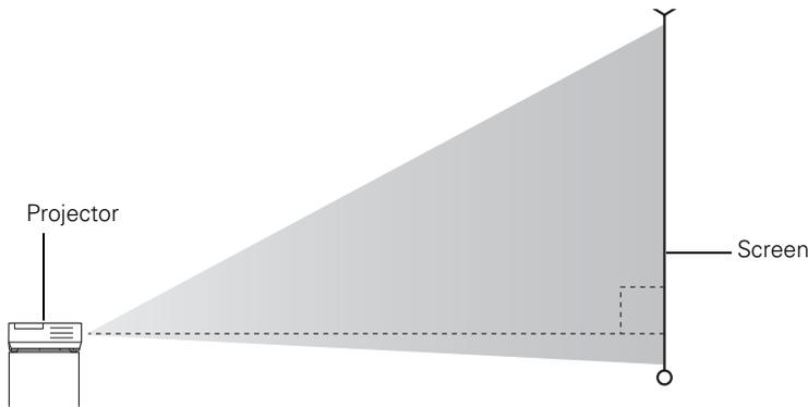
If you place the projector below screen level, you'll have to tilt it up by extending the front adjustable foot. This causes the image to become “keystone” shaped, but you can correct the distortion by pressing the buttons on the projector. See page 23 for detailed information about correcting the image shape.
