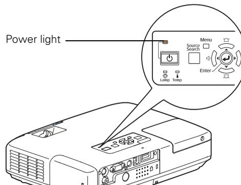
3. Press the red
